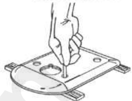
Figure 34. Removing a Worn Plate Roller Shell
